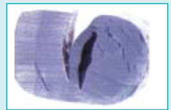
O-Ring with explosive decomposition damage
